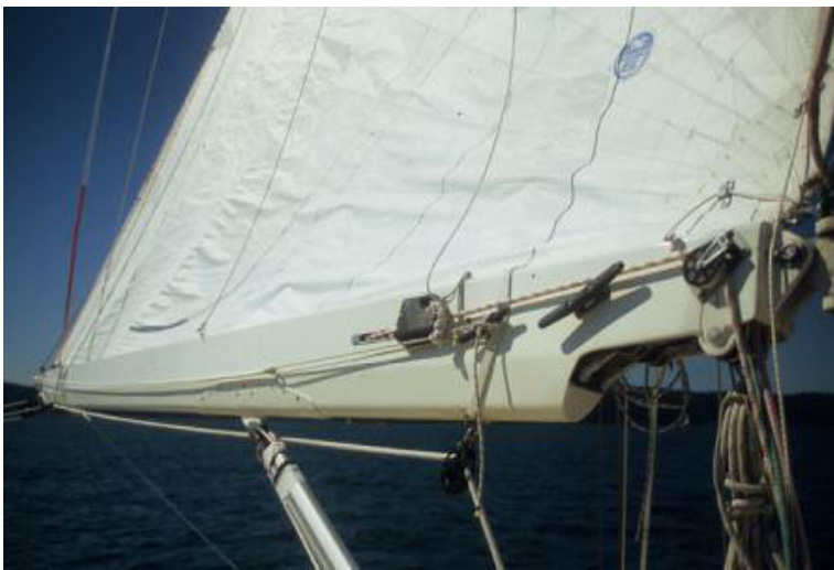
Preventer stowed on boom
