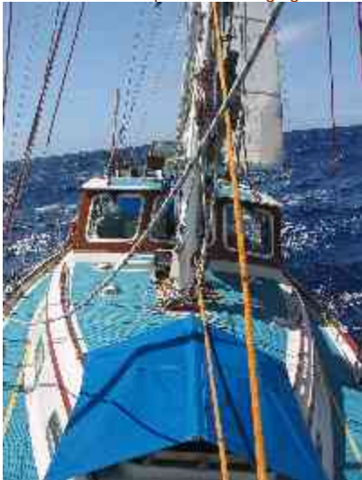
Orange downhaul over the winch and hatch. Outhaul falls and preventer hanging down.
