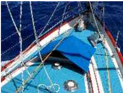
Orange downhaul over the winch and hatch. Outhaul falls and preventer hanging down.
